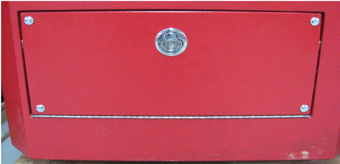
Diagram 1.12: QLM door permanently secured with 4 bolts .
